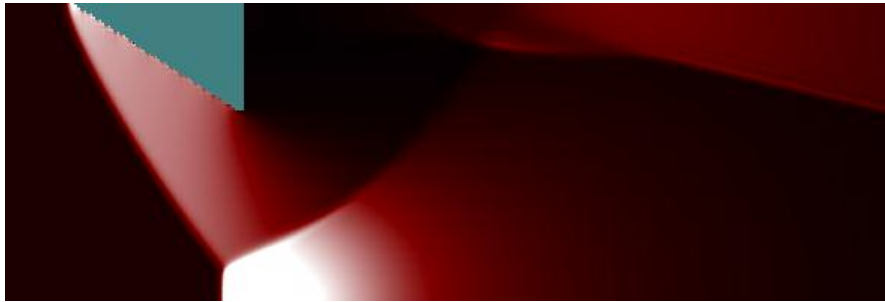
Fig. 2 Pressure Distribution for Supersonic Flow Around a Wedge with Mach Reflection
