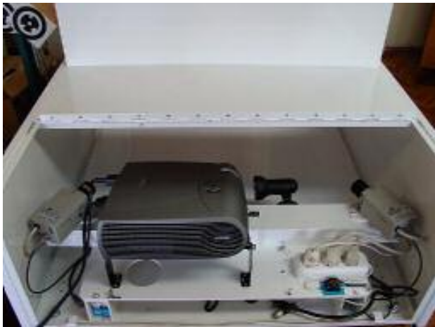
Figure 1: The exterior view of photogrammetric 3D reconstruction system.
